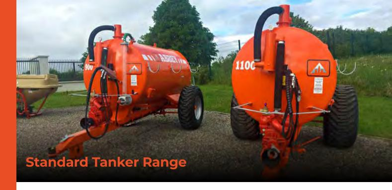
Standard Tankers range from 4,710L (1,100 gal) to 9,120L (2,000 gal). Produced to the highest standards, Tankers include heavy duty barrels, collared dish ends (for improved barrel strength and support), Battioni Pagani pumps, heavy duty axles and patented double trap pump protection system.
