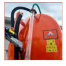
**LEVEL INDICATORS:** Sight Glass to indicate the end of Jlling. 100mm Front Level Indicator to show the volume of slurry when the tanker is Jling and emptying.
