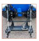
**REAR HYDRAULIC LINKAGE:** The linkage allows for the quick release and disconnection of the applicator from the linkage, leaving the rear mounted hydraulic linkage frame available to recouple to another Abbey
