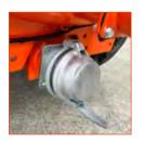
**STONE TRAP:** Stone trap with bauer coupling. Located at the base of the Tanker at the rear below the barrel of the Tanker to catch any unwanted stones and other debris.
