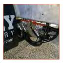
**DIVERTER:** Provides a simple solution to reduce the number of tractor hydraulic services needed to power multiple functions on a tanker.
