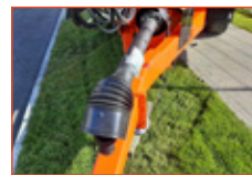
H: Wide Angle PTO Shaft (T80) With shear bolt protection.
