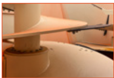
G: Mixing Auger Three vertical 22mm heavy duty augers to ensure perfect blend.
