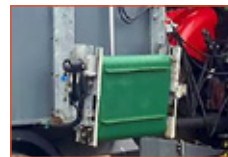
F: Discharge Conveyors Hydraulic discharge conveyors can be fitted to side door model vertical feeders to allow feed into bunkers.
