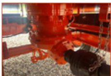
I: Corner Gearbox Uniquely integrated to the auger for better stability, protection and two speed gear box.
