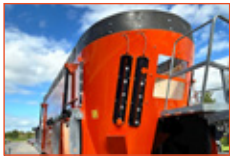
A: Tri-Auger Tub Tubs are 33.5m 3 .
