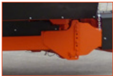
C: Independent Chassis Electronic scales with six weigh bars.
